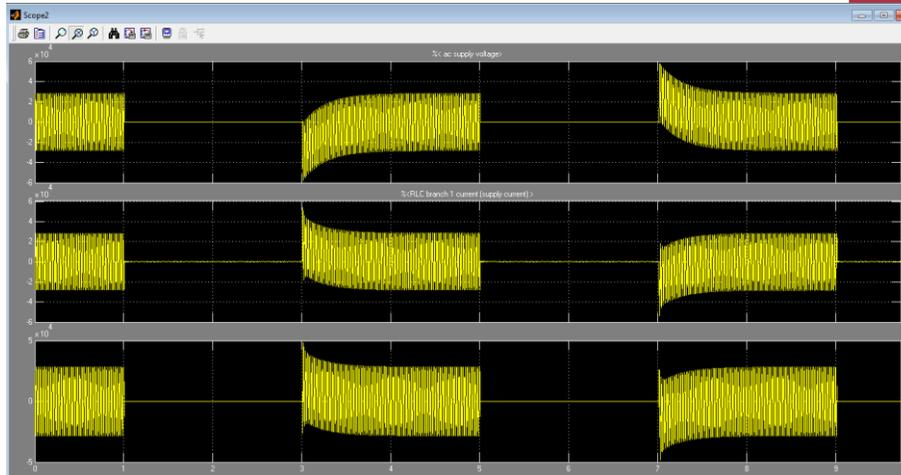
**Figure 5: Voltage stresses across the breaker poles (maximum stress touches 58 kV)**
