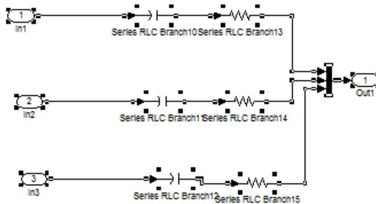
**Figure 1(c): Snubber circuit (subsystem 1 and 2)**
