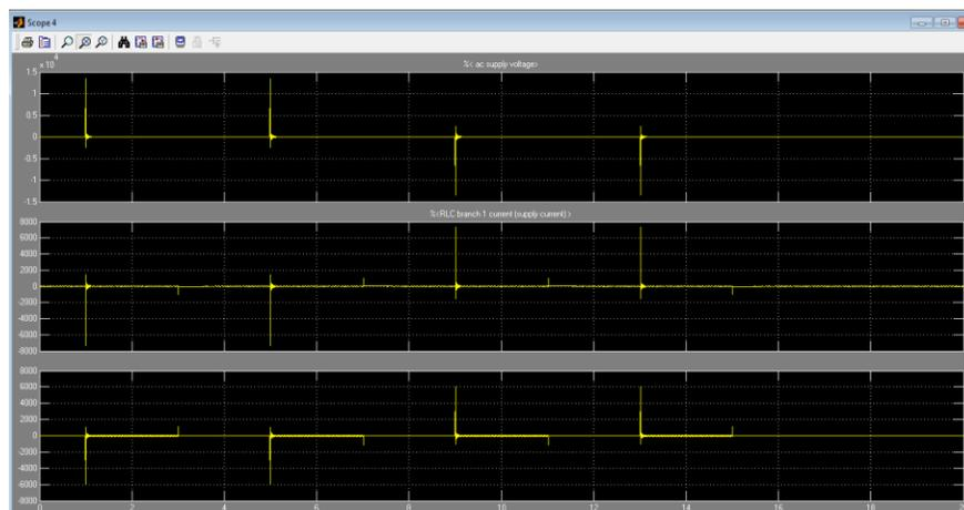
**Figure 8: Voltages across the 0.2% inrush current reactors “with” the parallel resistor of 24 Ω**
