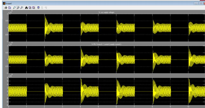
**Figure 3 (b): Voltage stresses across the breaker poles (maximum stress touches 84 kV)**
