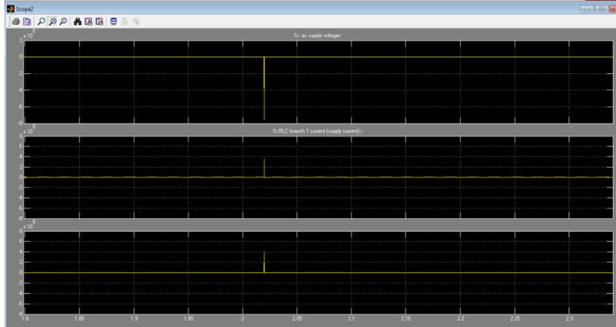
**Figure 2 (d): Voltage stresses across the breaker poles, expanded view of fig. 2(c ) (maximum stress touches nearly 770 MV)**
