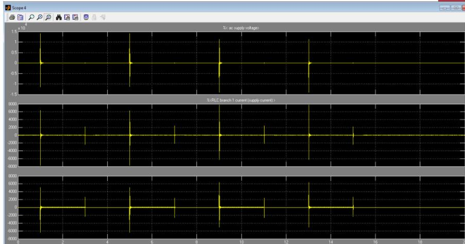
**Figure 7: Voltages across the 0.2% inrush current reactors “without” the parallel resistor of 24 Ω**
