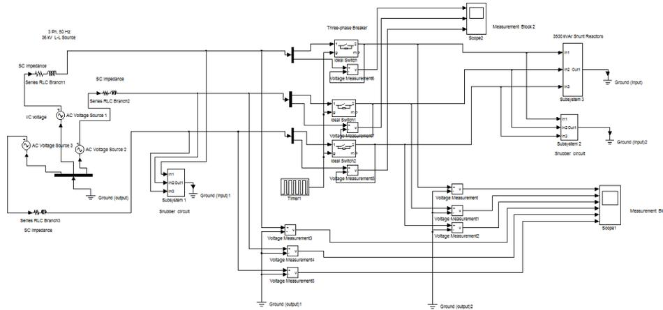
**Figure 1: Matlab model for the 36 kV substation reactors and breaker**
