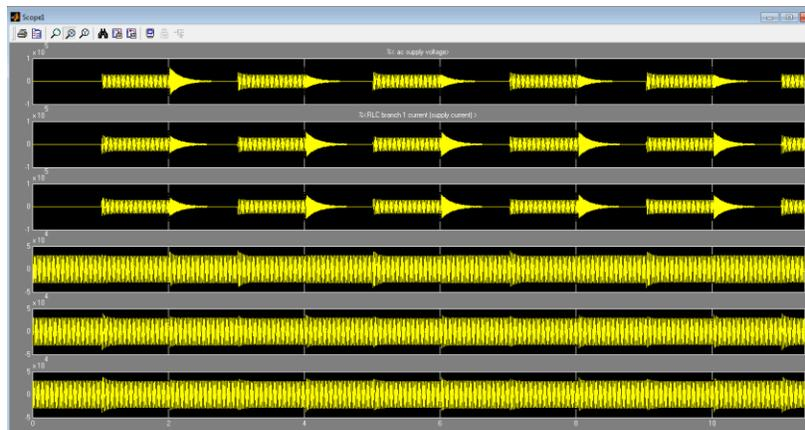
**Figure 3 (a): Voltage stresses for the breaker poles (output to neutral and input to neutral)**
