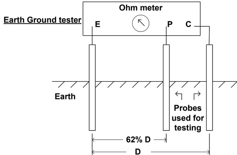
**Figure 2: Earth resistance measurement**
