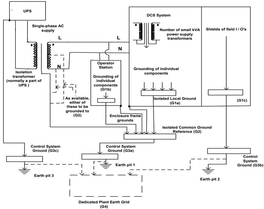
**Figure 4: Grounding and earthing scheme for Distributed Control Systems**
