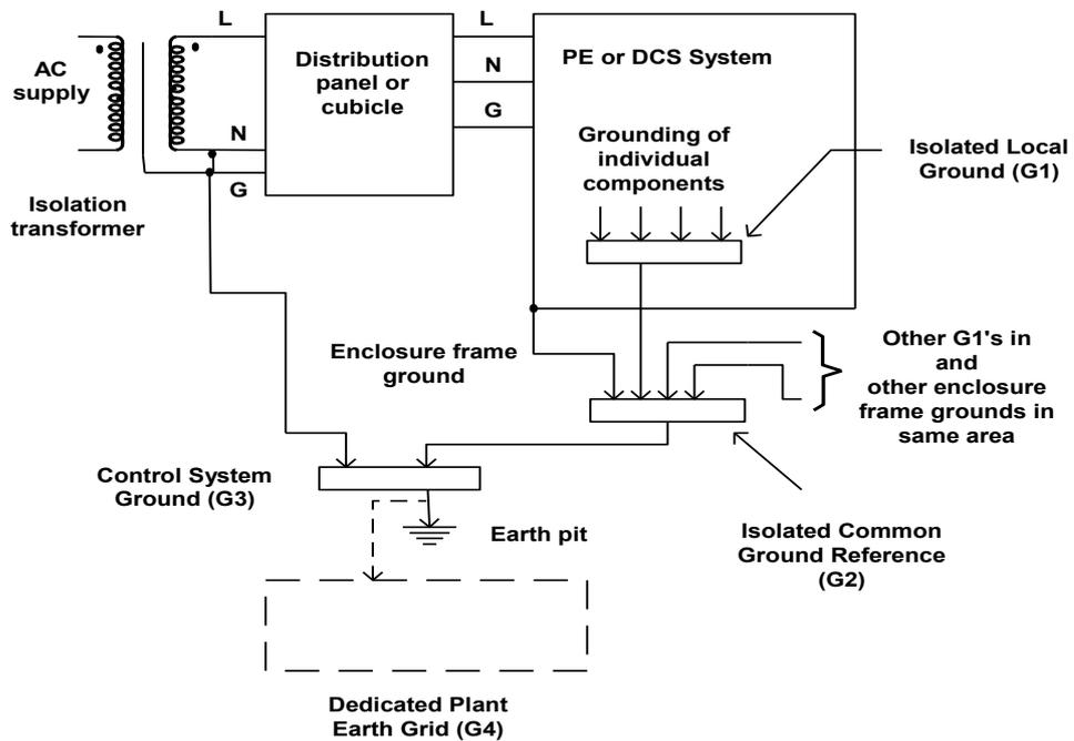
**Figure 3: Typical distribution system with grounding and earthing definitions**
