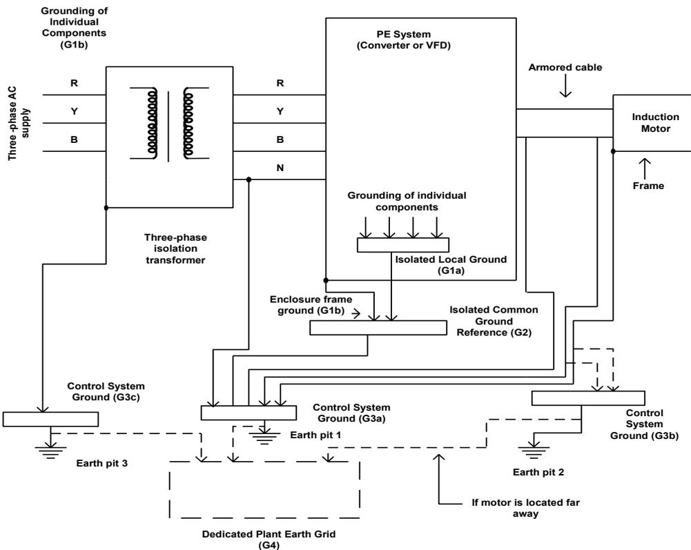
**Figure 5: Grounding and earthing scheme for Power Electronic Systems**
